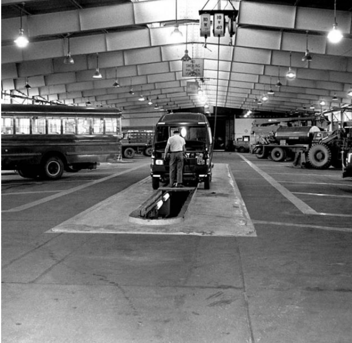
A worker of the 52 Transportation Squadron prepares to work on a van positioned over a grease pit at the maintenance shop.
